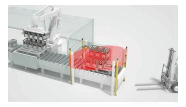
Solution: The loading area of the conveyor line is safeguarded at both the entry and exit side by multiple light beam safety devices. The area between the photoelectric sensors is monitored for the presence of persons by means of safety radar sensors.
